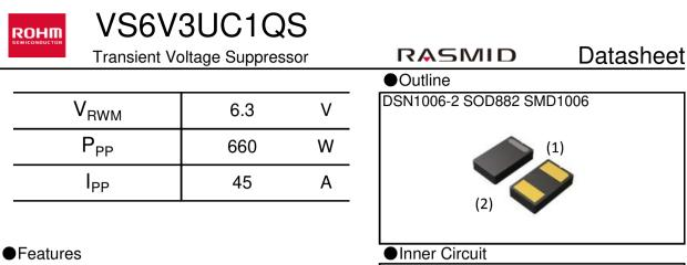
High reliability Uni-directional ESD protection ESD protection ±30kV (IEC61000-4-2) Dimension tolerance±10um
