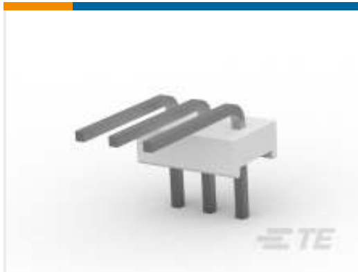
TE Part #640457-5 PCB Header: Polyester, Right Angle, Unshrouded
