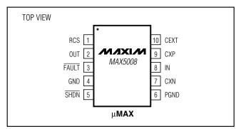
low-impedance trace, and connect the ground for  $C_{IN}$ ,  $C_{EXT}$ , and  $C_{OUT}$  directly to PGND in a star configuration. Connect  $R_{CS}$  to  $C_{EXT}$  through a short and low impedance trace.
