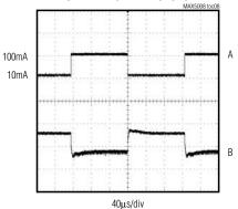
A: LOAD CURRENT B: OUTPUT VOLTAGE: AC-COUPLED, 100mV/div
