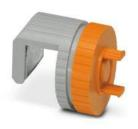
The optional holding device ensures the Rogowski coil is securely seated on busbars that are 5 ... 10 mm thick. During installation, the coil housing is pushed onto the flange of the holding device and snaps in automatically.
