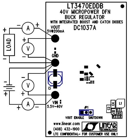
INSTALL SHUNT AT JP1: PINS 1&2=VOUT ENABLE PINS 2&3=SHUT DOWN
