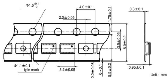
Note) Feed holes might be cover with the adhesive tape, but nothing will affect for using by that.
