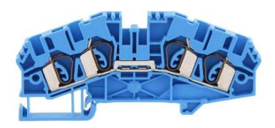
Feed-through terminal, Tension-spring connection, Mounting type: Mounting rail TS 35/7.5, Rated cross-section: 4 mm², Width: 6.1 mm, Colour: Blue
