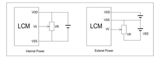
VDD-V0: LCD Driving Voltage VR: 10k-20k
