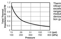
Thermal impedance reduces significantly with pressure, ensuring excellent performance in pressure ranges common for most standard modules and power electronic devices per manufacturer's application guide.
