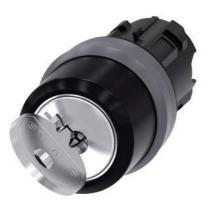
RONIS key-operated switch, 22 mm, round, plastic with metal front ring, lock number 455, with 2 keys, 2 switch positions O-I, latching, actuating angle 90°, 10:30h/13:30h, key removal O, with laser labeling, upper case and lower case, always upper case at the beginning of the word
