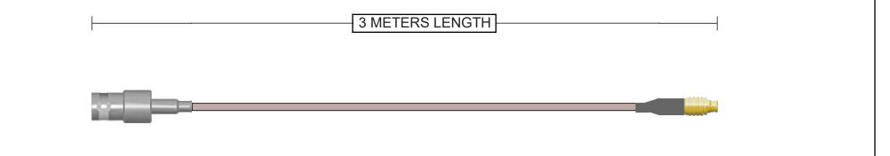
Connector A 112160 BNC Jack Straight Brass Nickel 50 Ohm RG-316 Continuity/Hi-Pot Connector B SMP-FS-C08-1-R SMP Plug Straight Beryllium Copper Gold + Heatshrink
