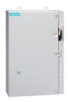
Non-reversing motor starter Size 0 Three phase full voltage Solid-state overload relay OLRelay amp range 5.5-22A 240V 50HZ / 277V 60HZ coil Combination type 25Amp circuit breaker Encl NEMA type 4X 316 S-steel Water/dust tight noncorrosive Extra-wide enclosure
