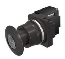
30mm BlackMax, Epoxy Coated Corrosion Resistant Complete Metal Unit Illuminated Push-Pull Operator Transformer type, 480V AC Incandescent Lamp Mushroom Head Cap Small 1 3/4" (44.5 mm) Metal, Black with Clear Lens 3 Position Pull-Momentary/Push-Maintained UL Listed, CSA Certified NEMA 1,3,3R,4,4X,12,13 & Automotive Standards
