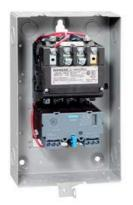
Non-reversing motor starter Size 1 Single phase full voltage Solid-state overload relay OLRelay amp range 0.75-3.4A 110-120/220-240VAC 60HZ coil Combination type Indoor general purpose use
