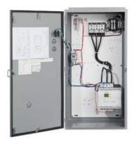
Enclosed soft starter, Controller 3RW44356BC34, Std. duty rating 75HP @460V, Std. duty current rating 117A Control voltage 115Vac Enclosure type NEMA 3/3R Weather proof outdoor use
