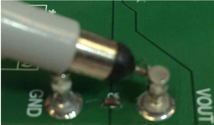
Figure 3. Output Ripple Measurement Technique
