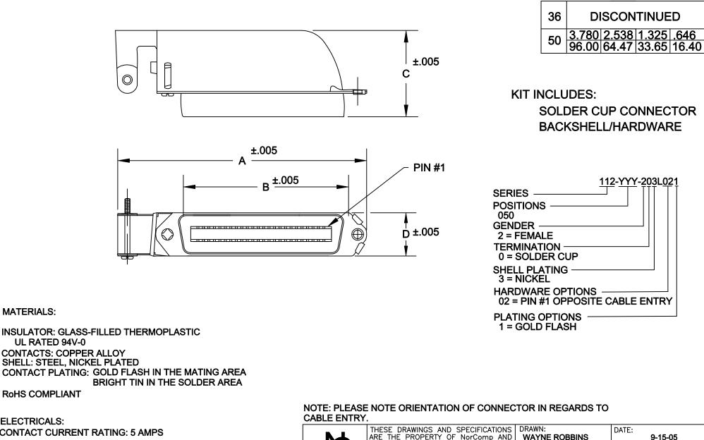
**ELECTRICALS: CONTACT CURRENT RATING: 5 AMPS** DIELECTRIC WITHSTANDING VOLTAGE: AC 1200 R.M.S. INSULATION RESISTANCE: 1000 mohms MINIMUM AT 500V DC **CONTACT RESISTANCE: 30 mOHMS MAXIMUM** OPERATING TEMPERATURE: -55°C TO +125°C
