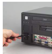
Plug ring-lock securely fastens the power cord
