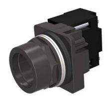
30mm BlackMax, Epoxy Coated Corrosion Resistant Complete Metal Unit Illuminated Push-Pull Operator Full Voltage, 6V AC/DC Incandescent Lamp Less Mushroom Head Cap 3 Position Momentary UL Listed, CSA Certified NEMA 1,3,3R,4,4X,12,13 & Automotive Standards
