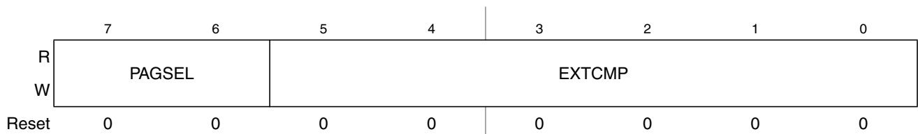
Figure 18-19. Debug Comparator B Extended Register (DBGCBX)
