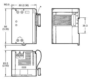
\*A flat cable with a length of 85 mm can be used.
