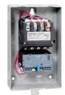
Non-reversing motor starter Size 1 3/4 Three phase full voltage Solid-state overload relay OLRelay amp range 10-40a 208VAC 60HZ coil Combination type Indoor general purpose use
