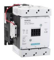
Vacuum NEMA contactor, Size 6, Three phase full voltage, Contactor amp rating 540A, 3 wire (NO aux included), 200-220V 50-60Hz/DC coil, Non-combination type, Enclosure NEMA type (open), No enclosure
