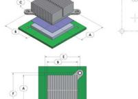
1) Dimension A is the length of the heat sink in the direction of the flow.
