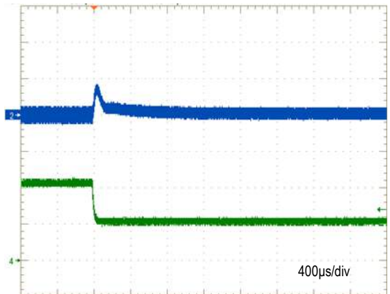
Transient Response (V in =48V, I out =2.125A to 1.06A, Ta=+25°C) Ch2=V out , 200mV/div, Ch4=I out , 1A/div
