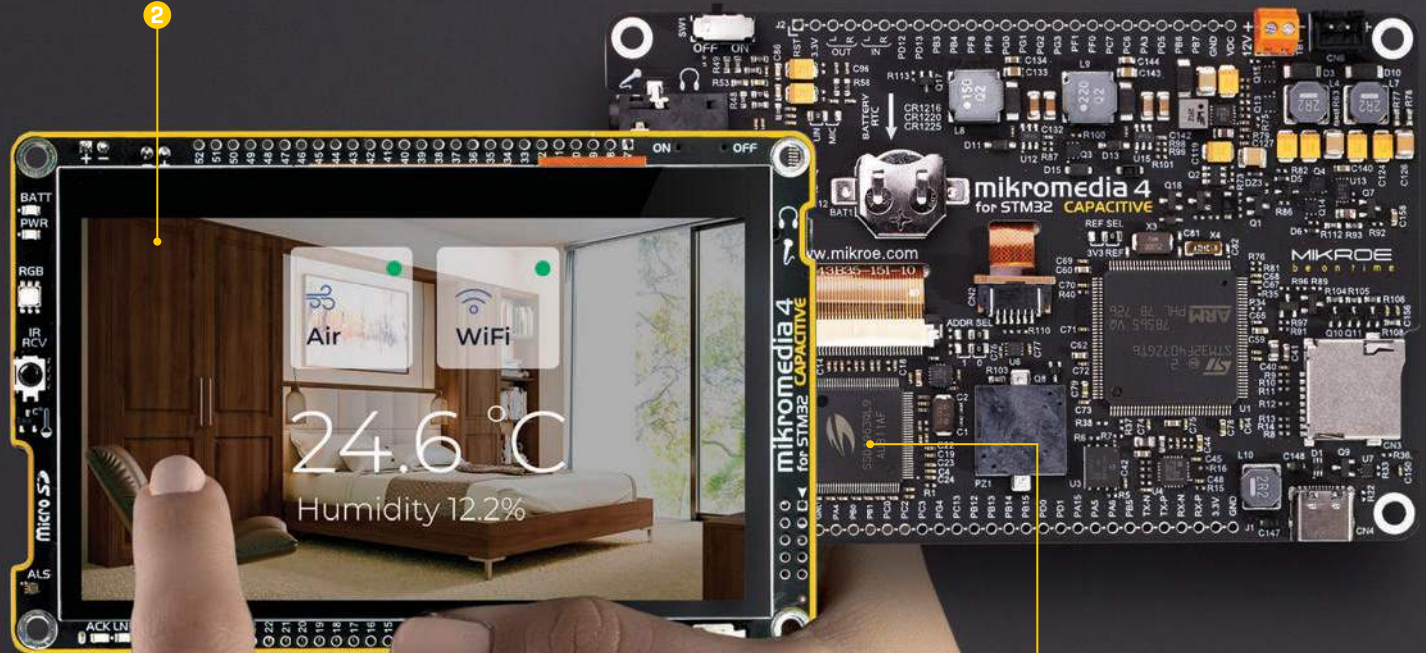
Figure 9: Display and SSD1963 view
