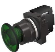
30mm BlackMax, Epoxy Coated Corrosion Resistant Complete Metal Unit Illuminated Push-Pull Operator Full Voltage, 24V AC/DC Incandescent Lamp Mushroom Head Cap Small 1 3/4" (44.5 mm) Plastic, Green 3 Position Momentary UL Listed, CSA Certified NEMA 1,3,3R,4,4X,12,13 & Automotive Standards
