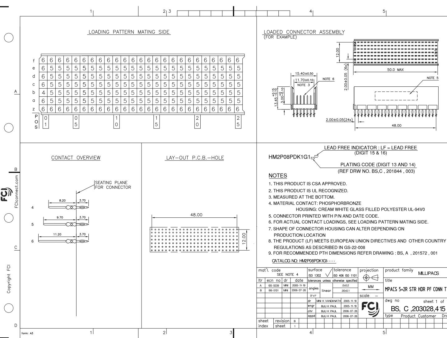
50.0 MAX NOTE 5 Α 48.00 LEAD FREE INDICATOR : LF = LEAD FREE (DIGIT 15 & 16) PLATING CODE (DIGIT 13 AND 14) В (REF DRW NO. BS,C, 201844, 003) С product family projection MILLIPACS  $\bigcirc \bigcirc$ title ΜМ MPACS 5+2R STR HDR PF CONN TYPE B scale \_\_\_\_ dwg no sheet 1 of 1 |size| 5 FC BS. C .203028,415 Аз Y type Product Customer Drawing D
