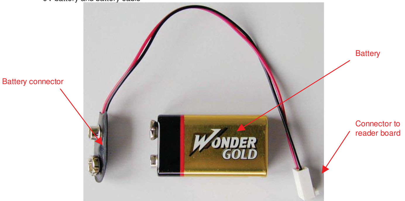
Figure 4 The 9V battery and the power supply cable
