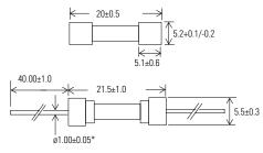
Note: \*Rating of 20A has 1.20±0.05 diameter lead ſ
