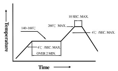
3. DIP soldering (Wave Soldering):
