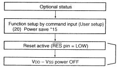
Set the time (t) from reset active to turning off the VDD - Vss power (VDD - Vss = 1.8 V) longer than the time ( $t_H$ ) when the potential of  $V_5 \sim V_1$ becomes below the threshold voltage (approximately 1 V) of the LCD panel. For th, refer to the <Reference Data> of this event. When th is too long, insert a resistor between Vs and VDD to reduce it.
