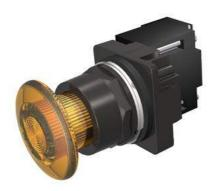
30mm BlackMax, Epoxy Coated Corrosion Resistant Complete Metal Unit Illuminated Push-Pull Operator Transformer type, 480V AC LED Lamp Mushroom Head Cap Small 1 3/4" (44.5 mm) Plastic, Amber 3 Position Momentary UL Listed, CSA Certified NEMA 1,3,3R,4,4X,12,13 & Automotive Standards
