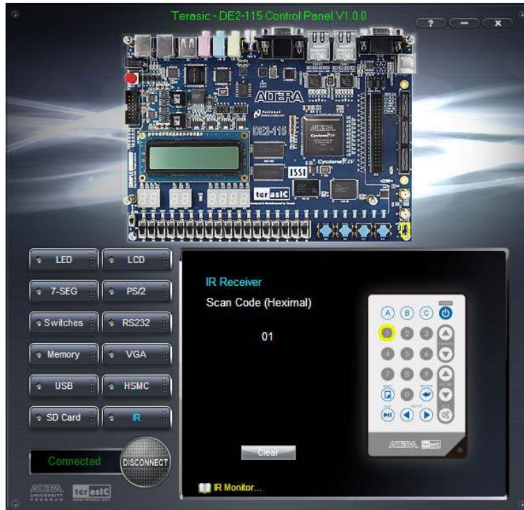
Figure 3-14 Testing the IR receiver using remote controller
