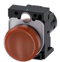
Indicator lights, compact, 22 mm, round, plastic, amber, lens, smooth, with holder, Operating voltage 24 V AC/DC, screw terminal
