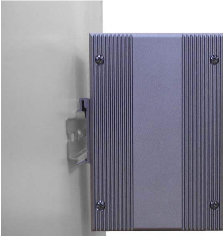
Figure 2.3-3 Installation to DIN-rail Step 2
