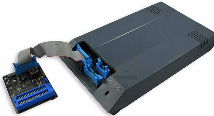
Figure 5. OTP Programming Adapter (Included with Crimson ICE)
