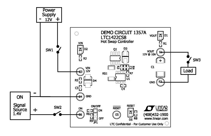
Figure 1. Proper Measurement Equipment Setup
