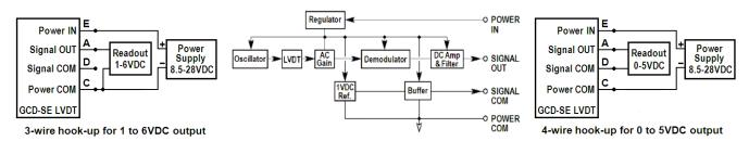
A through E: Connector pin assignments
