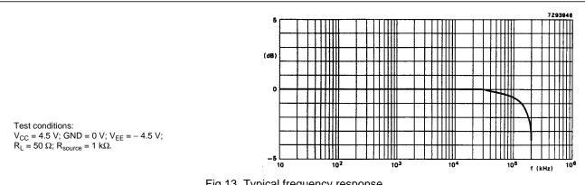
Fig.13 Typical frequency response.
