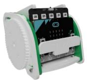
**STEP 4:** Secure the SERVO:LITE board and micro:bit with the :MOVE T-piece.
