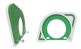
**STEP 5:** Attach to the chassis, slot the nut into the T-joint and tighten the screw.
