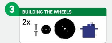
**STEP 1:** Screw the 2 larger screws from the servo packet, through the wheel and into the appropriate holes in the servo attachment. The centre of the horn and the centre of the wheel should be aligned. Press fit the wheel onto the servo and repeat for the opposite side.
