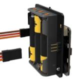
**STEP 1:** Plug the servo cables back into the SERVO:LITE board. The left servo should plug into the left-hand side of the :MOVE board and vice versa. The cables should be threaded down the gaps on either side as shown and any excess tucked under the pen mounting plate.
