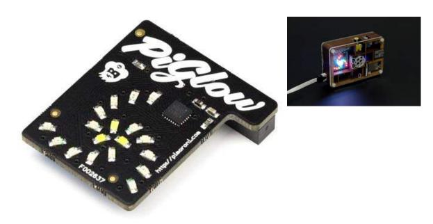
The PiGlow is a small add on board for the Raspberry Pi that provides 18 individually controllable LEDs. You can use it for all sorts of things! And of course, it fits inside a Pibow!
