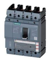
circuit breaker 3VA5 UL frame 250 breaking capacity class C 100kA @ 480V 4-pole, line protection TM210, FTFM, In=225A overload protection Ir=225A fixed short-circuit protection Ii=10 x In N conductor unprotected without connection
