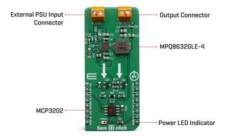
The output voltage is determined by the feedback voltage on the FB pin. The output voltage is set to 3.3V making it usable with most embedded applications, allowing them to be powered from the same source, like the rest of the application, which may use a higher voltage for its operation. This is a common-case scenario in various field applications where a relatively high voltage is required i.e. for servos, step motors, displays, etc.
