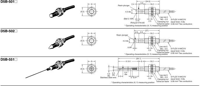
Note: 1. Unless otherwise specified, a tolerance of ±0.4 mm applies to all dimensions.
