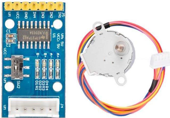
The Gear Stepper Motor Driver Pack includes a stepper motor and a motor drive board. It's a four-phase eight-stepping stepper motor, and you can easily control this stepper motor via the drive board.
