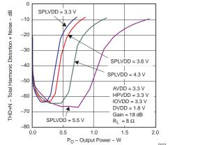
Figure 4-9. Total Harmonic Distortion + Noise vs Output Power Class-D Speaker-Driver Output Power
