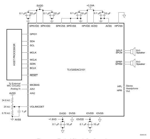
Figure 7-1. Typical Circuit Configuration
