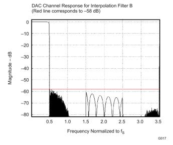
Figure 6-14. Frequency Response of Channel Interpolation Filter B
