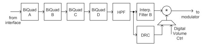
Figure 6-5. Signal Chain for PRB\_P8 and PRB\_P13
