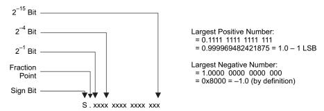
Figure 6-12. 1.15 2s-Complement Coefficient Format
