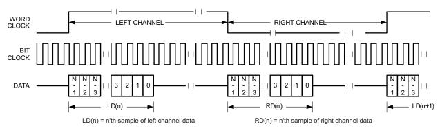
Figure 6-24. Timing Diagram for Left-Justified Mode
