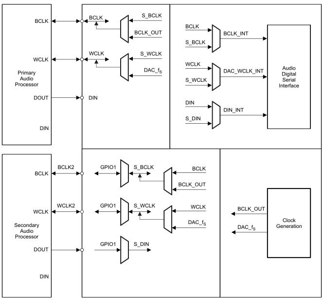
Figure 6-33. Audio Serial Interface Multiplexing
