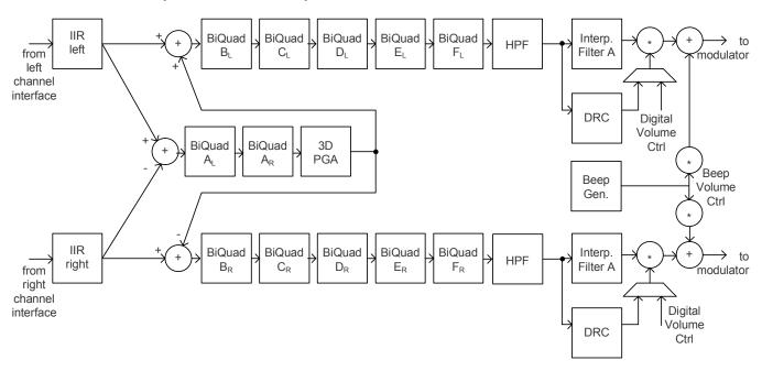
Figure 6-11. Signal Chain for PRB\_P25
