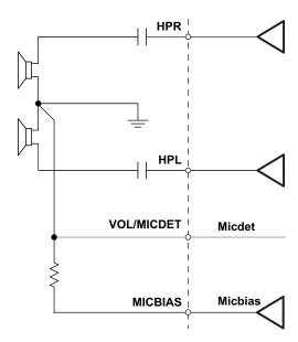
Figure 6-17. Jack Connections for Headphone Detection
