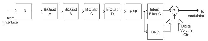
Figure 6-7. Signal Chain for PRB P18 and PRB P21
