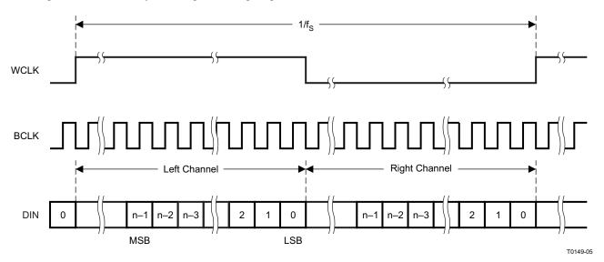
Figure 6-23. Timing Diagram for Right-Justified Mode
