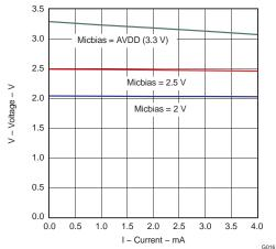
Figure 4-12. Voltage vs Current MICBIAS
