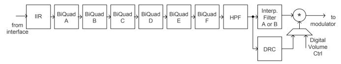
Figure 6-2. Signal Chain for PRB\_P2, PRB\_P5, PRB\_P10, and PRB\_P15
