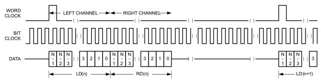
Figure 6-32. Timing Diagram for DSP Mode With Offset = 0 and Bit Clock Inverted
