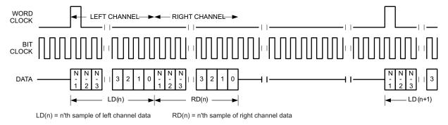
Figure 6-30. Timing Diagram for DSP Mode
