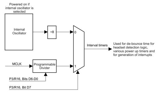
Figure 6-22. Interval Timer Clock Selection
