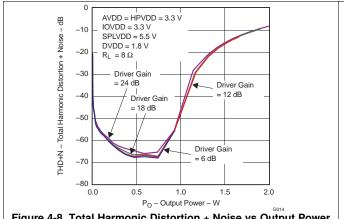
Figure 4-8. Total Harmonic Distortion + Noise vs Output Power Max Class-D Speaker-Driver Output Power
