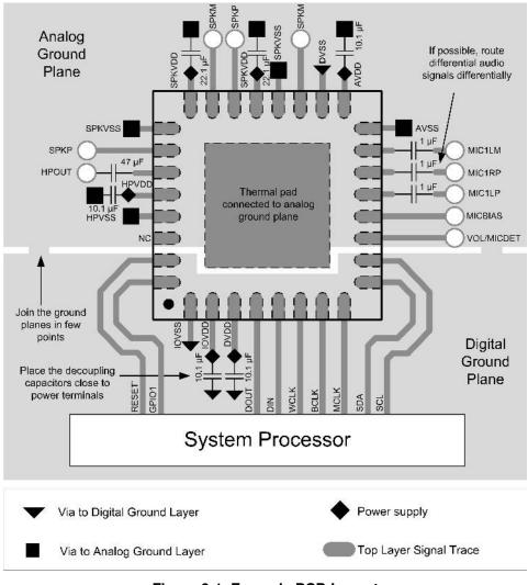
Figure 9-1. Example PCB Layout
