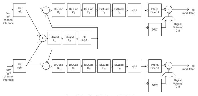
Figure 6-10. Signal Chain for PRB\_P24
