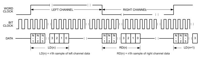
Figure 6-26. Timing Diagram for Left-Justified Mode With Offset = 0 and Inverted Bit Clock
