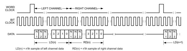
Figure 6-31. Timing Diagram for DSP Mode With Offset = 1
