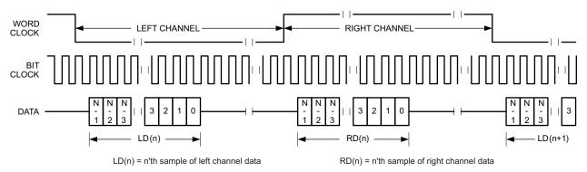
Figure 6-29. Timing Diagram for I<sup>2</sup>S Mode With Offset = 0 and Bit Clock Inverted
