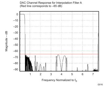
Figure 6-13. Frequency Response of DAC Interpolation Filter A
