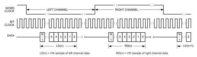
Figure 6-28. Timing Diagram for I<sup>2</sup>S Mode With Offset = 2
