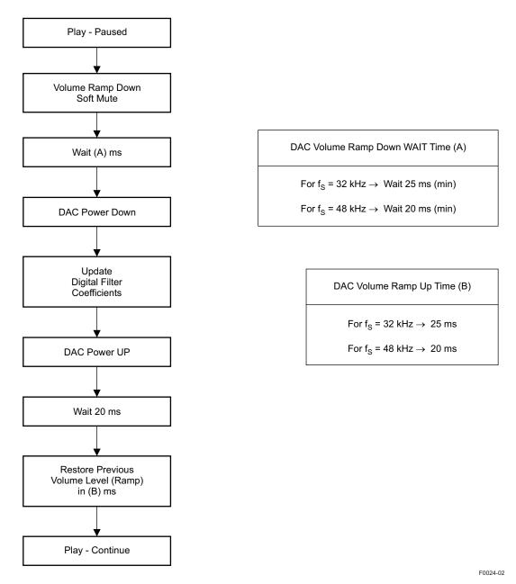
Figure 6-18. Example Flow For Updating DAC Digital Filter Coefficients During Play
