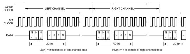
Figure 6-27. Timing Diagram for I<sup>2</sup>S Mode
