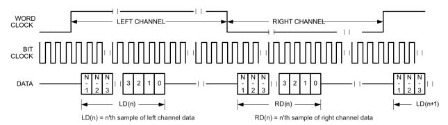
Figure 6-25. Timing Diagram for Left-Justified Mode With Offset = 1
