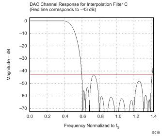
Figure 6-15. Frequency Response of DAC Interpolation Filter C
