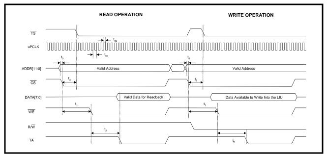
TABLE 7: INTEL MICROPROCESSOR INTERFACE TIMING SPECIFICATIONS
