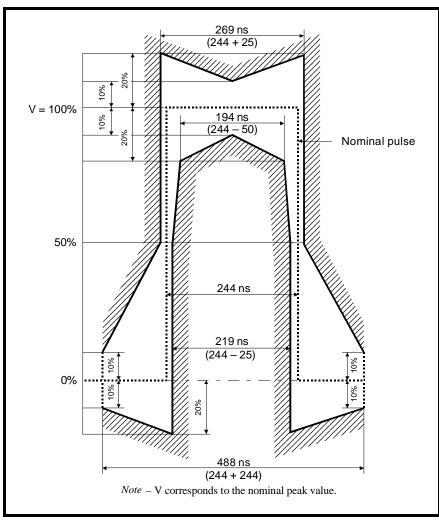
FIGURE 120. ITU G.703 PULSE TEMPLATE
