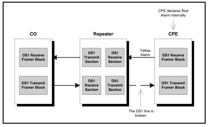
The Repeater, upon detection of Yellow Alarm originated from the CPE, will transmit a Blue Alarm, also known as Alarm Indication Signal (AIS) to the CO. Blue alarm is an all ones pattern indicating that the equipment is functioning but unable to offer service due to failures originated from remote side. It is sent such that the equipment downstream will not lose clock synchronization even though no meaningful data is received. The
