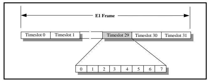
Not all of these timeslots are available to transmit voice or user data. For instance, timeslot 0 is always reserved for system use and timeslot 16 is sometimes used (reserved) by the system. Hence, within each E1 frame, either 30 or 31 of the 32 timeslots are available for transporting user or voice data. In general, there are two types of E1 frames, FAS and Non-FAS. In any E1 data stream, the E1 frame begins with a FAS frame followed by Non-FAS frame and then alternates between the two.
