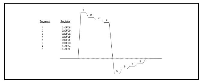
**Note:** By default, the arbitrary segments are programmed to 0x00h. The transmitter outputs will result in an all zero pattern to the line interface.
