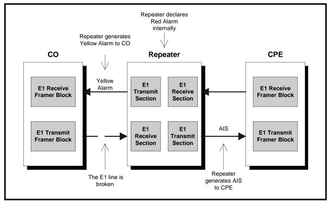
Now, the CPE uses the AIS signal sent by the Repeater to recover received clock and remain in synchronization with the system. Upon detecting the incoming AIS signal, the CPE will generate a Yellow Alarm automatically to the Repeater to indicate the loss of incoming data. Figure 100 below illustrates this scenario in which the Repeater is sending an AIS to the CPE and the CPE is sending a Yellow Alarm back to the Repeater.
