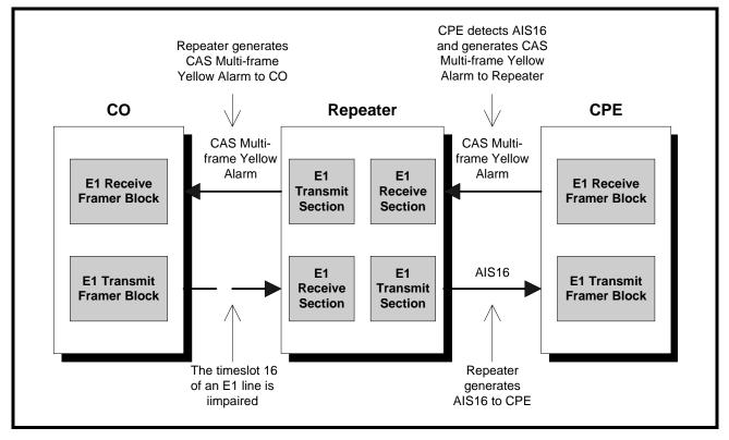
In summary, AIS or Blue Alarm is sent by a piece of E1 equipment downstream indicating that the incoming signal from upstream is lost. Yellow Alarm is sent by a piece of E1 equipment upstream upon detection of Loss of Signal, Loss of Frame or when it is receiving AIS.
