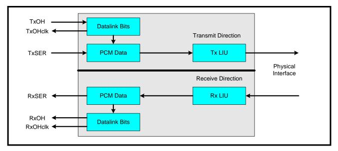
FIGURE 20. T1 EXTERNAL OVERHEAD DATALINK BUS
