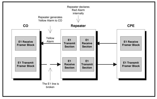
The Repeater will also transmit a Blue Alarm, also known as Alarm Indication Signal (AIS) to the CPE. Blue alarm is an all ones pattern indicating that the equipment is functioning but unable to offer service due to failures originated from remote side. It is sent such that the equipment downstream will not lose clock
