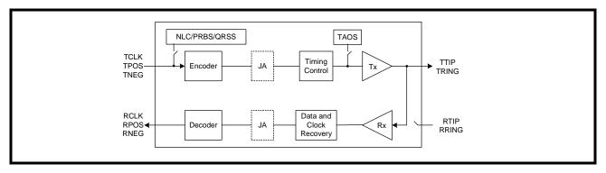
**Note:** The transmit diagnostic features such as TAOS, NLC generation, and QRSS take priority over the transmit input data at TCLK/TPOS/TNEG.
