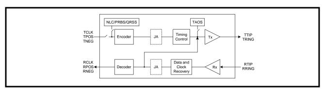
FIGURE 28. SIMPLIFIED BLOCK DIAGRAM OF REMOTE LOOPBACK
