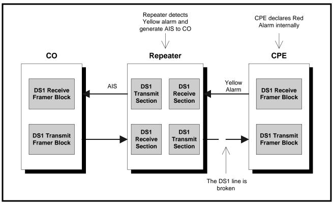
Now let us consider another scenario in which the DS1 line between CO and the Repeater is broken. Again, upon detection of Loss of Signal (LOS) or Loss of Frame (LOF) condition, the Repeater will generate an internal Red Alarm. This alarm will normally trigger a microprocessor interrupt informing the user that an incoming signal failure is happening.
