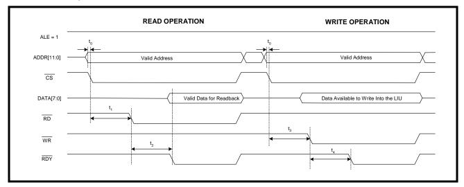
TABLE 6: INTEL MICROPROCESSOR INTERFACE TIMING SPECIFICATIONS
