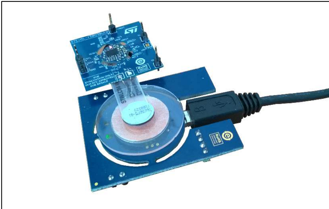
Figure 25: Transmitter – receiver setup with UART cable
