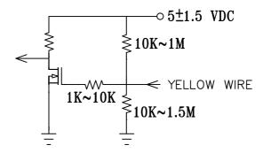
13-1. THE FAN SPEED WILL DEFAULT TO MAXIMUM WHEN THE SPEED CONTROLL INPUT IS LEFT UNCONNECTED.
